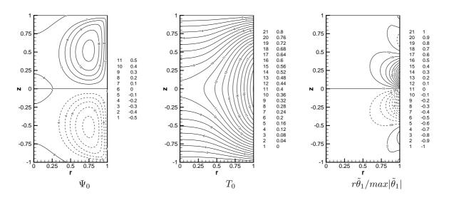
The stream function  $\Psi_0$  and temperature  $T_0$  are represented for the steady flow at Ma = 106, the critical Marangoni number being equal to 104.4. The temperature component of the first adjoint eigenmode, normalized and multiplied by r, is displayed on the right. The application of a temperature impulse has maximal efficiency when it is applied on the free surface near the mid plane.
